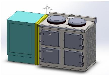
If you want to bring the cupboards closer, then you must ad insulation about 75mm thick. We recommend a material called calcium silicate boards which is very effective and we can supply 100cm by 90cm boards. These are 30mm thick.
