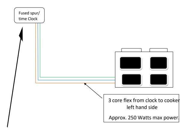
Fused spur/clock with 5-amp fuse. Connect to ring main and leave a flex cable down to the LHS of the cooker.
