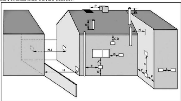
Please Note where the terminal is within 1 metre of any plastic material, such material should be protected from the effects of the combustion products of the fuel.
